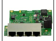
Embedded format, takes up minimal space, with mounting holes connected to Functional Earth
