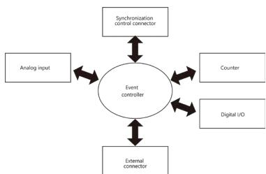
Scenario 1: Connect two devices with synchronization control connector, synchronize with analog input of one device, and perform analog input of the other device.
