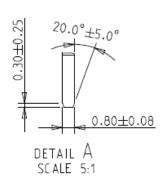
TOLERANCE: ±0.15mm UNIT: mm
