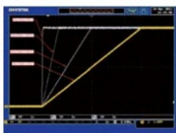
The Adjustable Rise Time of the PSW 30V Module
