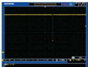
Momentary drop in supply voltage by ASR-2000 Series
